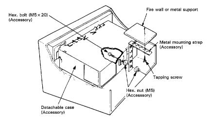
■ To install in the Japanese car, fix using the 2 of the holes indicated with ● with TP screw (M5).
